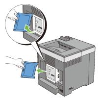
4 Align the connector of the memory module with the slot, and insert the memory module into the slot.
